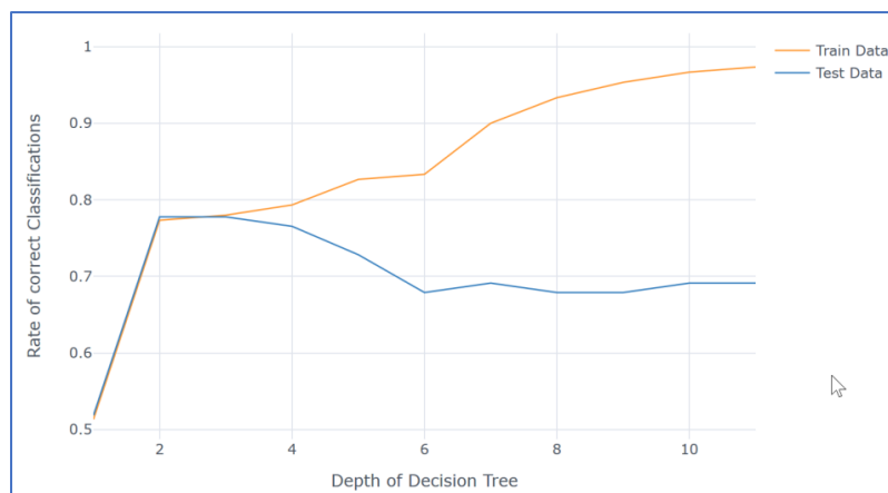
Figure 2. Evolution of rate of correct classifications during the training process of a decision tree (Visualization from the Basic ProDaBi Decision Tree JNB )
