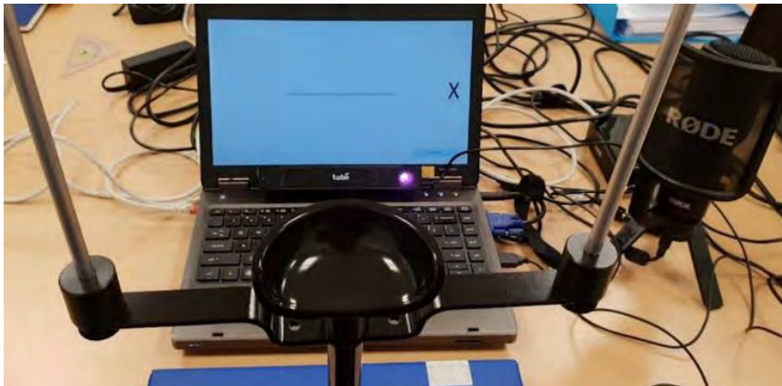
Figure A.1 Set up of the laptop, Tobii eye-tracker, chin rest and microphone
