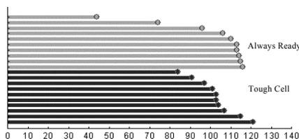
Figure 4. The Life Span of Two Brands of Batteries
